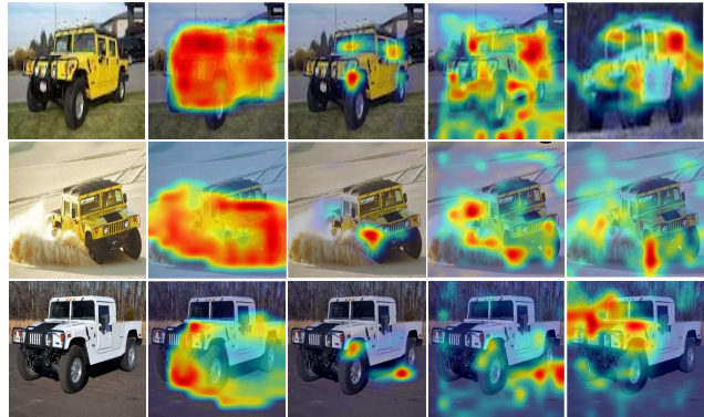
Figure 5. Visualisation of learned convolutional feature maps from Cars dataset with ResNeXt-101 backbone. From left: Input image, GAP, iSQRT-COV, Precision Matrix and iSICE.
